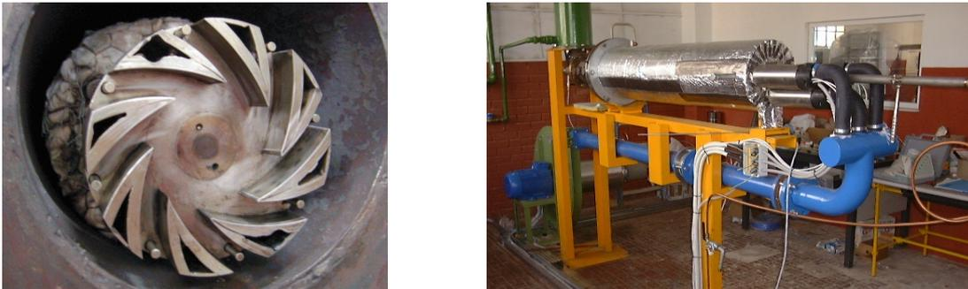
*Fig. 1 LRPM radially-inward swirler and burner test-rig*
